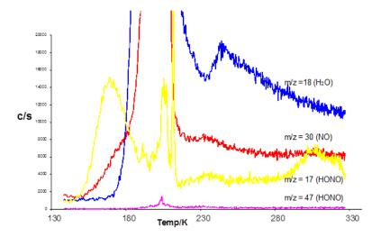
Thermal Desorption Profiles obtained on the Hiden Mass Spectrometer of  $NO_y$  and  $H_2O$  subsequent to photolysis of  $D_{2h}$ - $N_2O_4$  in water ice. The mass spectral signal m/z=17 has been corrected for the contribution from water using the water fragmentation pattern 74% m/z=18, 17% m/z=17.
