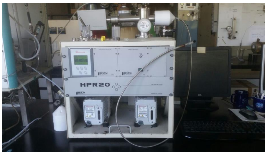
The Hidden HPR-20 EGA in the Lab used for characterisation and testing of catalytic samples
